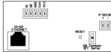
IOLAN DS1 A4D2 – 4 Analog inputs and 2 Digital I/O and 1 RS-232/422/485 Serial Port
