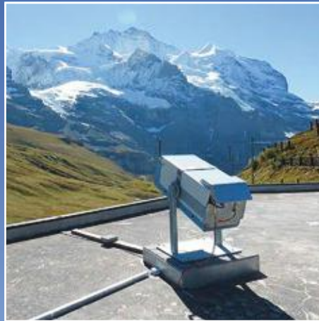
Equipment is required on location to check the functionality. The Lufft cloud height simulator allows ceilometers to be tested, even under a cloudless sky.
