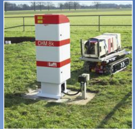
Ceilometers are often of dual use – for airport weather information and meteorology.
