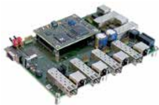
Example of Embedded Ethernet Switch EES25 on development kit
